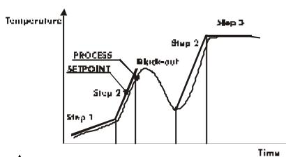
Cycle recovery is particularly useful for firing plants. After a black-out, the controller ATR420 can restart the cycle from the point at which it was interrupted. The gradient will be the same of the running step.
