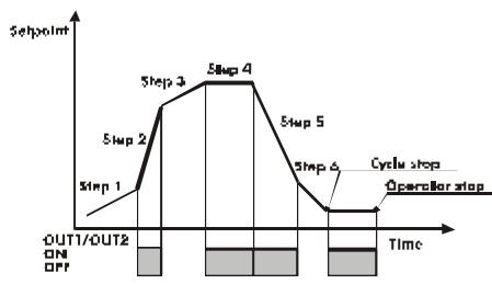
ON- or OFF-state of auxiliary output can be selected for each step of the cycle. State is selectable also at cycle end. See 5.1.
