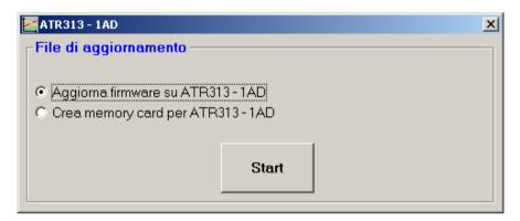
Select choosen option (upgrade firmware or create memory card). **START** keys allows to visualize a mask for the entering of path and name of upgrade file.
